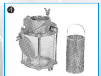
Clean the filter and the cylinder or replace them if necessary
