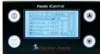
iControl panel for i-Series generators
